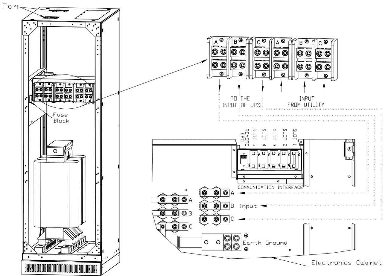
**Figure 6 – Input Transformer Cabinet 208/480V**
