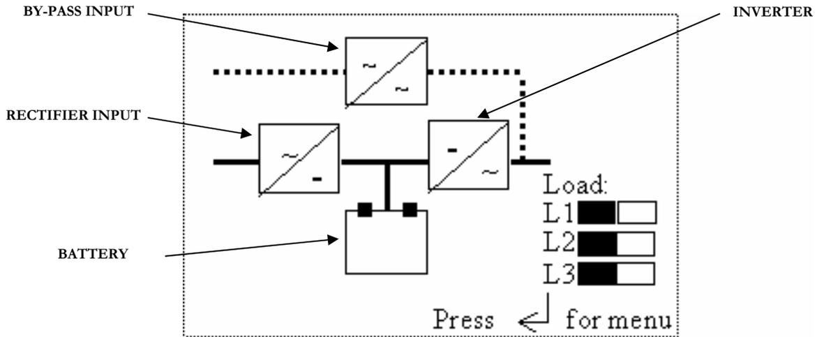
13 LCD Screen – Shows graphical and functional parameters
