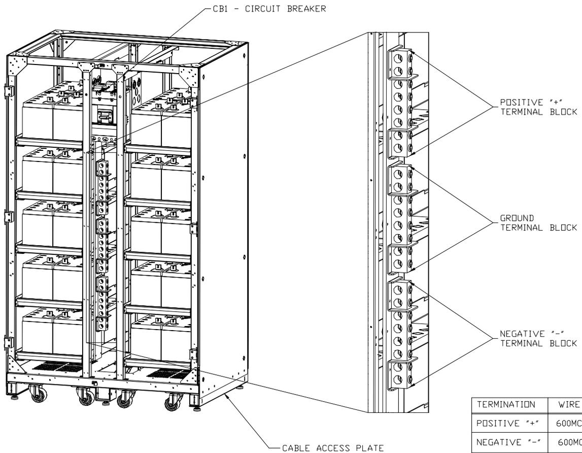
**Figure 8 – Battery Cabinet Electrical Connections**
