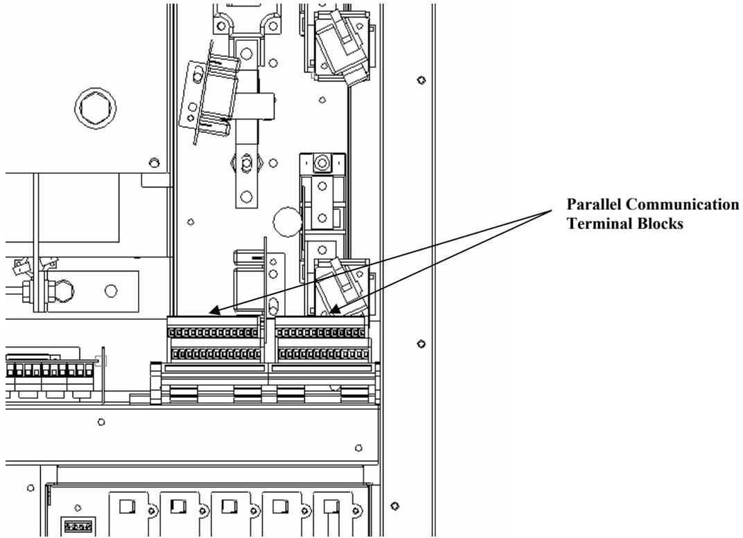
**Fig 14- Parallel Communication Terminal Blocks Location**
