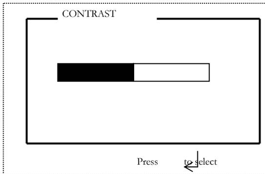
22 The **Contrast** screen is used to adjust the contrast of the display for ease of readability. Use the left and right arrow to adjust the contrast of the screen. To return to previous screen, press ESC button.
