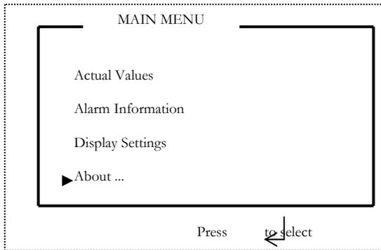
23 The **Main Menu** screen's function is to provide the user the selection options for viewing various information about the UPS. This is the highest level for menu. To return to previous screen, press ESC button. Press the ENTER button to select screen. Use the UP and DOWN arrows to toggle through current screen. (Shown for About sub menu)
