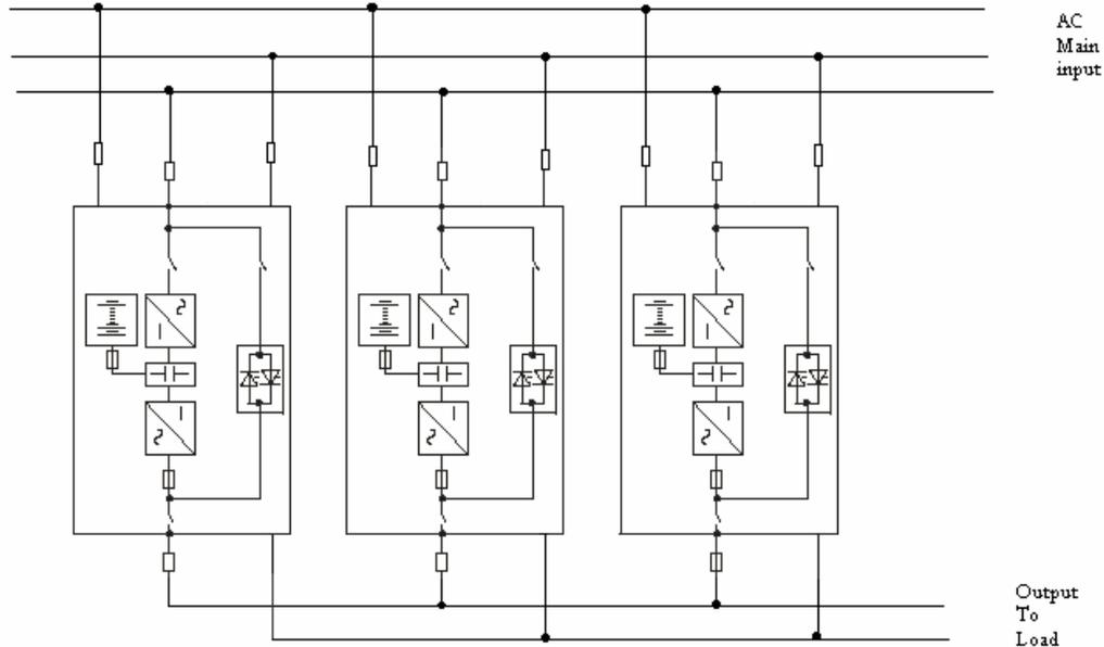
**Fig 11- Parallel Configuration**
