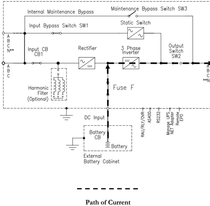
In Battery operation, the On Battery and Summary Alarm LEDs on the control panel are illuminated. If an overload condition occurs at the output, the UPS switches to By-pass operation, if available.
