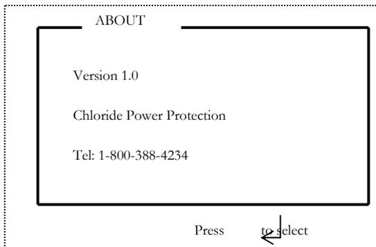
24 The **About** screen shows the software revision, manufacturer and support information including the hotline. To return to previous screen, press ESC button.
