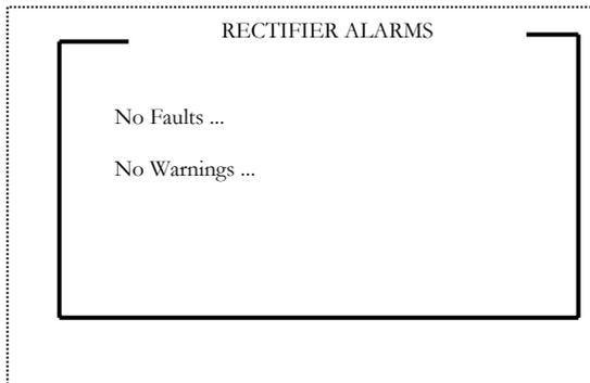
16 The **Rectifier Alarms** information screen displays parameters regarding the alarms. (Shown for No Faults and No Warnings) To return to previous screen, press ESC button.
