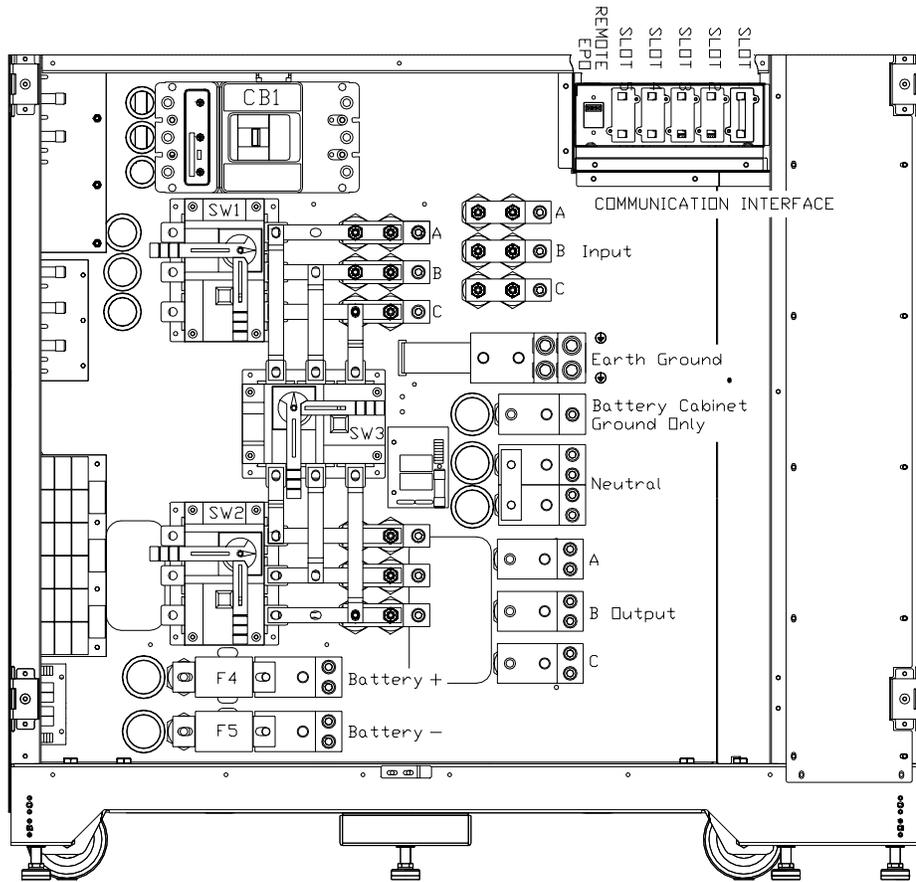
**Figure 5 – UPS Electrical Terminations**
