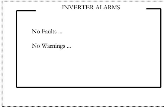
13 The **Inverter Alarms** information screen displays parameters regarding the alarms. (Shown for No Faults and No Warnings) To return to previous screen, press ESC button.
