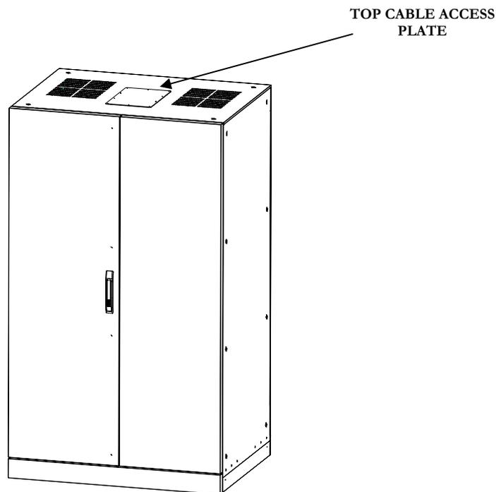
*Figure 7 – Battery Cabinet Top Cable Access Plate*
