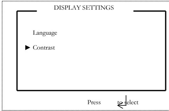
21 The **Display Settings** screen displays sub menus regarding display settings. The display sub menus displayed are: *Language and Contrast*. To return to previous screen, press ESC button. (Shown for the Contrast sub menu)
