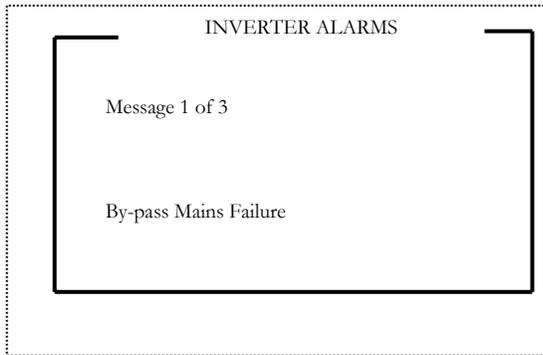
14 The **Inverter Alarms** Information screen is showing message 1 of 3 and specific information on alarm. Using the cursor will display any active alarm messages. To return to previous screen, press ESC button.
