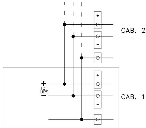
**Figure 9 – Multiple Cabinet Connections**
