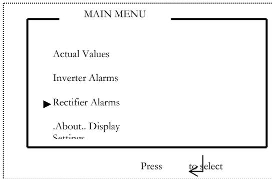
15 The **Main Menu** screen's function is to provide the user the selection options for viewing various information about the UPS. This is the highest level for menu. To return to previous screen, press ESC button. Press the ENTER button to select screen. Use the UP and DOWN arrows to toggle through current screen. (Shown for Rectifier Alarms)
