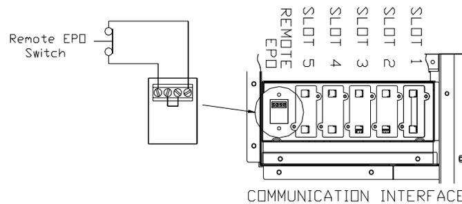
**Figure - 24 Remote Equipment Power Off (REPO)**
