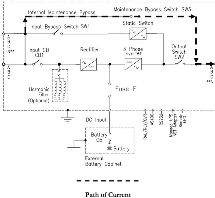
Note: In Maintenance By-pass operation, the Display and LED's do not illuminate.
