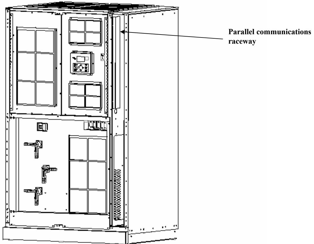
*Figure 13 – Raceway for Parallel Communication Wires*
