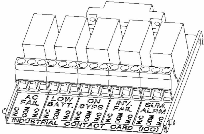
Figure - 22 Industrial Contact Card and Bracket
