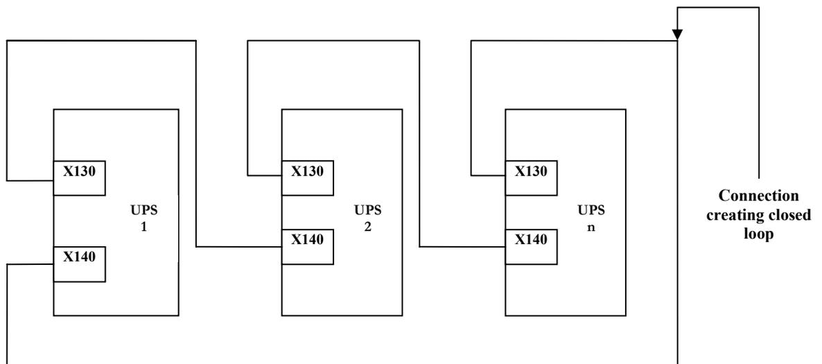
**Fig 12 - Parallel Communication Block Diagram. (Closed loop configuration)**
